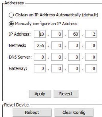
The screenshot shows the Dante Controller Network Config dialog box. It has two sections: 'Addresses' and 'Reset Device'. In the 'Addresses' section, the 'Manually configure an IP Address' radio button is selected. The fields are: 'IP Address' (10 . 0 . 60 . 2), 'Netmask' (255 . 0 . 0 . 0), 'DNS Server' (0 . 0 . 0 . 0), and 'Gateway' (0 . 0 . 0 . 0). There are 'Apply' and 'Revert' buttons. The 'Reset Device' section has 'Reboot' and 'Clear Config' buttons.
