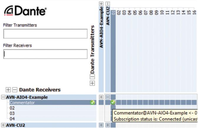
Fig 3-12: Simple Routing
