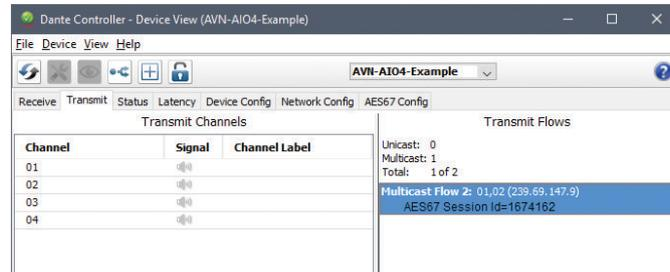
Fig 3-23: Multicast Flow in Side Pane
