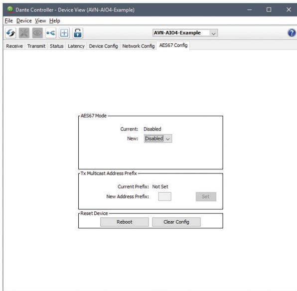
Fig 3-16: AES67 Config Tab with AES67 Mode Disabled
