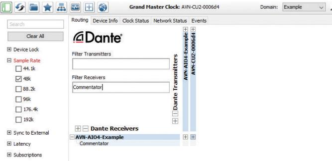
Fig 3-11: Filtering Channels
